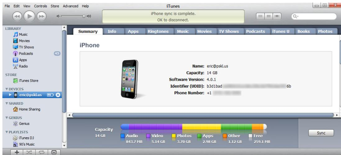
Figure 2: Apple's iTunes application, showing the attached phone's UDID.
